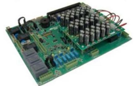
The board is fitted with a **DSP** microprocessor (**D**igital **S**ignal **P**rocessor) that reads line voltage, settings, motor currents and inputs and drives directly the motor by imposing direction and speed. On the basis of the motor current, the board also activates the protections against overload and short-circuit for the motor itself.
