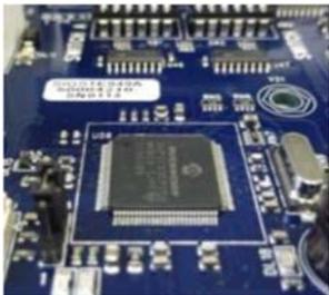
Using both microprocessors, the board reads line voltage, settings, motor currents and inputs then drives each motor directly by imposing direction and speed. On the basis of the motor current, the board also activates the protections against overload and short-circuit for the motor itself.
