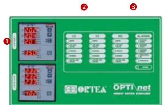
Any abnormal functioning generates an acoustic alarm that can be silenced by pressing the relevant button below the alarm LEDs.
